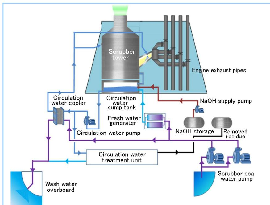
**Figure 3** Freshwater closed-cycle mode
