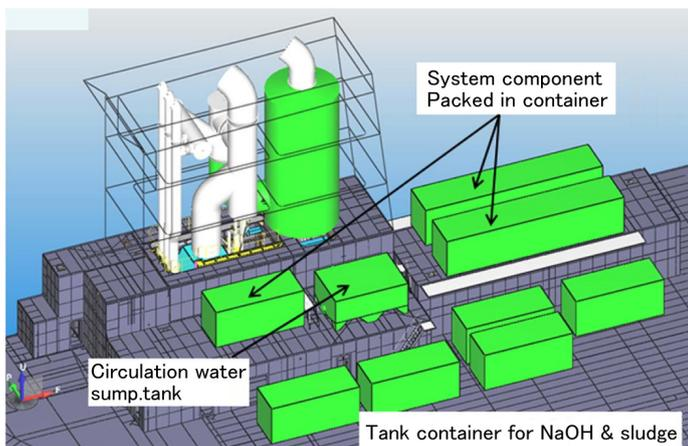
**Figure 6** Layout example of container-type module housing this system
