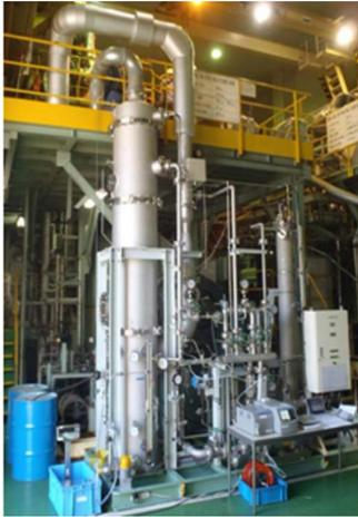
**Figure 1** SO<sub>x</sub> scrubber demonstration plant
