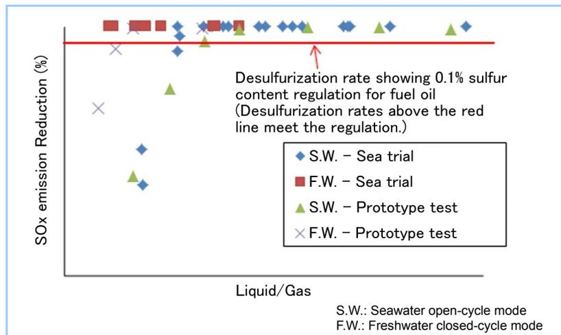
**Figure 9** FGD performance of the marine-use SO<sub>x</sub> scrubber system
