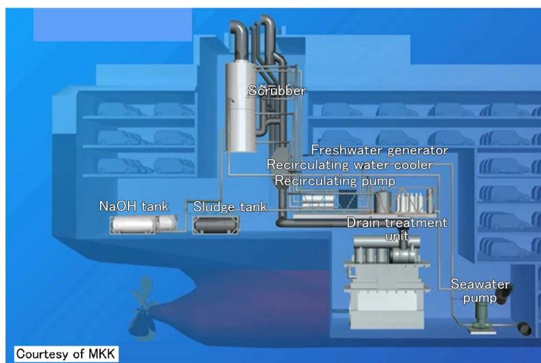
Figure 5 Example of system layout on a ship
