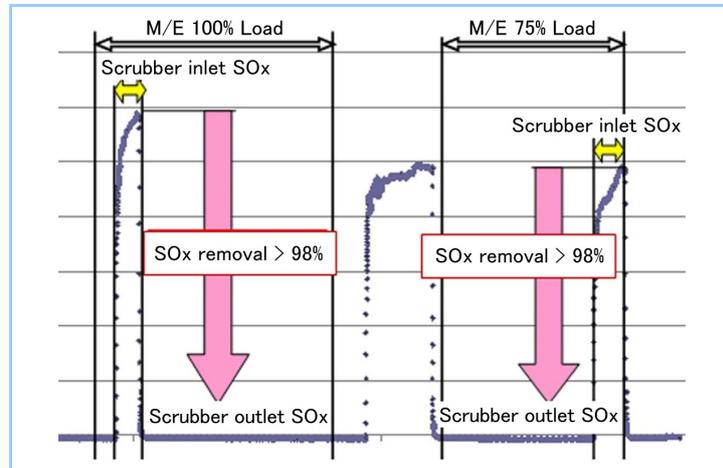
**Figure 2** Behavior example of SO<sub>2</sub> concentration at scrubber outlet at FGD test
