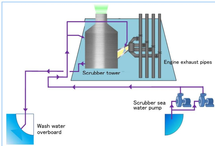
Figure 4 Seawater open-cycle mode
