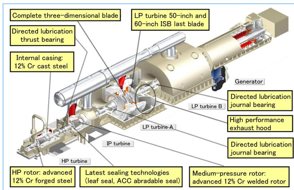
**Figure 5** Schematic view of 1000 MW tandem compound steam turbine and applied technologies
