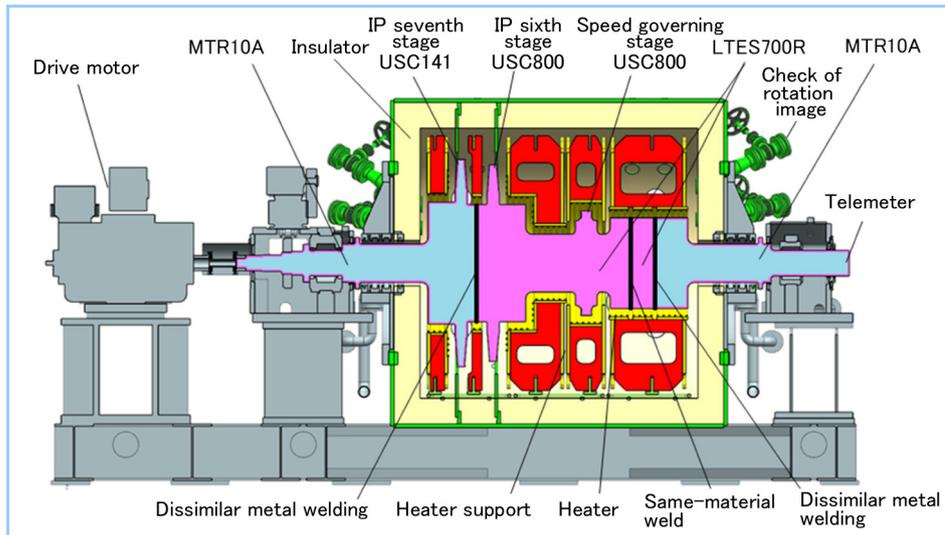
Figure 12 Rotor test facility and structure for rotation test
