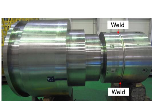
Figure 13 LTES700R welded rotor
