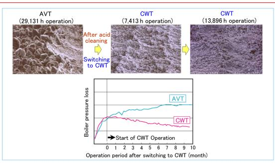
Figure 3 CWT effect of reduced rippled scale build-up
