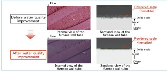
Figure 6 Powdered scale reduction via optimized water quality during normal operations
