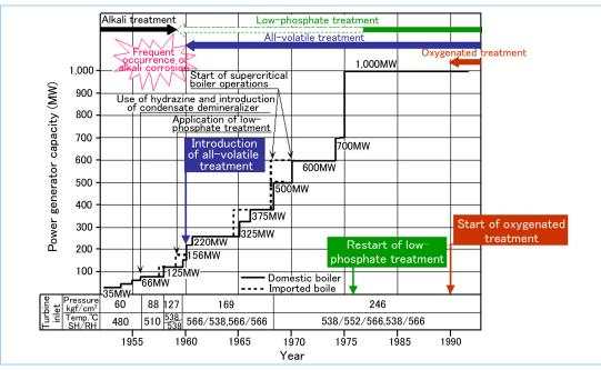
Figure 1 History of boiler feed-water treatment for domestic thermal power plants
