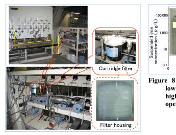
Figure 7 External view of the suspended iron removal test unit with a high-temperature filter for the low-pressure feed-water heater drain system
