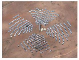
Figure 8 Plant image showing heliostat arrangement
