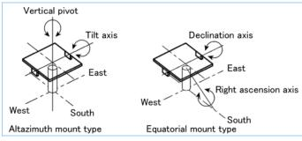
Figure 6 Examples of heliostat construction
