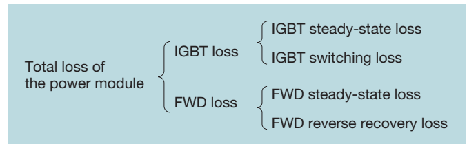
Fig. 3 Total power module losses The causes of power module loss are classified into four categories.
