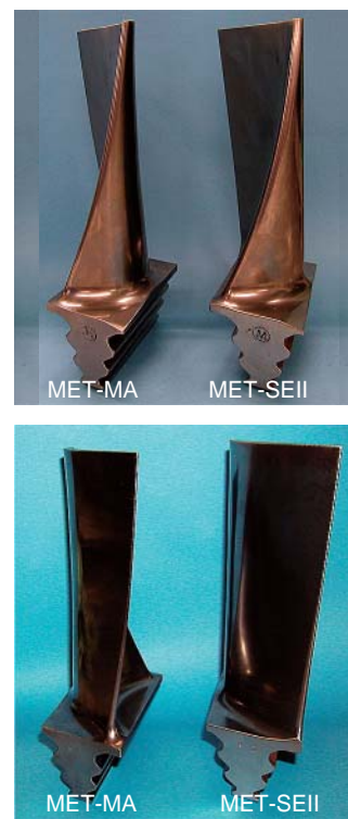
Fig. 5 External views of MET-MA and MET-SE II turbine blades
