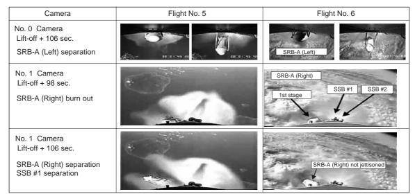
**Fig. 2 Photos by on board CCD cameras** The condition of rocket No. 6, whose SRB-A was not jettisoned, is shown as compared with that of rocket No. 5, whose SRB-As were jettisoned normally.
