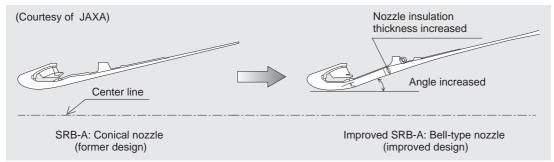
Fig. 4 Improvement of SRB-A nozzle The figure shows the improvements made to the SRB-A nozzle.
