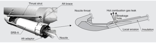
Fig. 3 Cause of the Flight No. 6 accident The figure shows the cause of the flight No.6 happened in the SRB-A nozzle.
