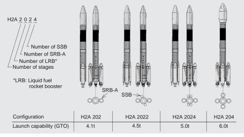
Fig. 1 H-IIA launch vehicle family This figure shows the H-IIA launch vehicle family
