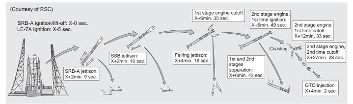
Fig. 7 Flight sequence of H-IIA Flight No.7
