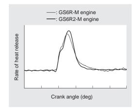
Fig. 4 Comparison of heat release rates The GS6R2-M engine has a shorter and more efficient combustion period.
