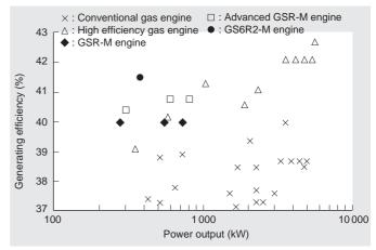
Fig. 2 Relation between generating efficiency and power output in the gas engine
