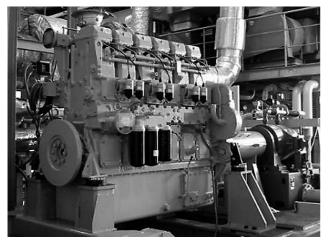
Fig. 1 External view of GS6R2 Miller cycle gas engine Prototype engine installed at the Osaka Gas Company. Joint performance tests and endurance tests were carried out on the engine.
