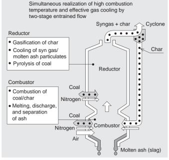
Fig. 6 Principle of air-blown gasifier
