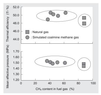
Fig. 12 Test results of simulated coal bed methane gas Indicates comparison of methane concentration in fuel, thermal efficiency, and output. Combustion performance of coalmine methane gas is equivalent to that of natural gas.
