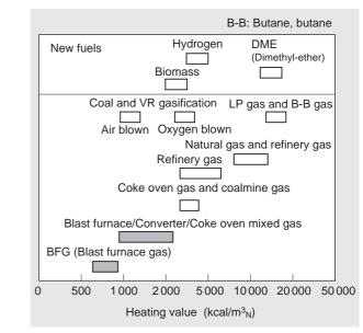
Fig. 8 Diversification of gas turbine fuels
