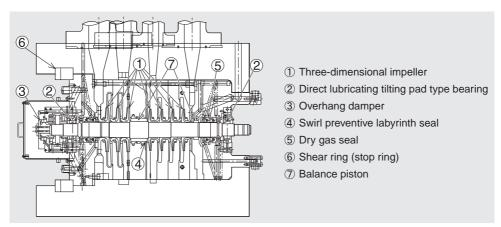
Fig. 2 A sectional view of CO<sub>2</sub> re-injection compressor Required advanced technology, and health, safety and environment protection features are shown in a sectional view of the  $CO_2$  re-injection compressor.
