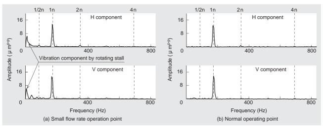
Fig. 5 Vibration characteristics (rotating stall occurrence point and normal operating point). Spectrum analysis result of rotor vibration. In small flow rate region, vibration at smaller than components of rotating speed (N) occurs due to rotating stall.
