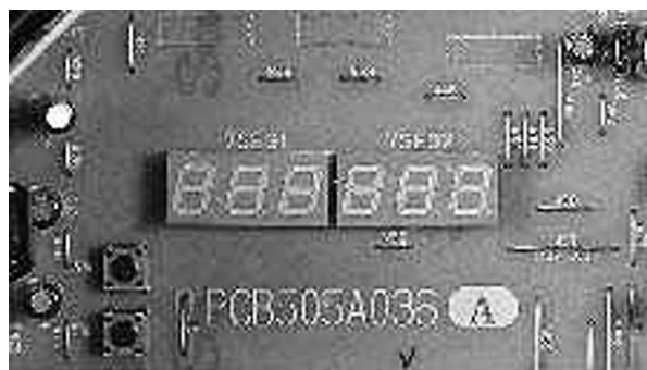
Fig. 7 Seven-segment display of outdoor controller
