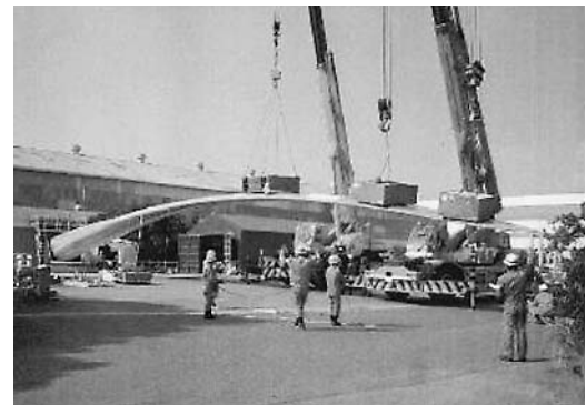
Fig. 6 Maximum load test of 29.5 m blade
