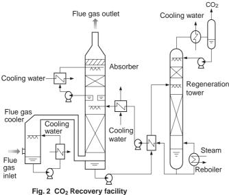
Flowchart of  $CO_2$  recovery from flue gas of boiler, etc.
