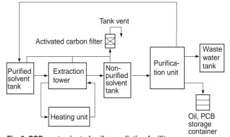
Fig. 3 PCB contaminated soil remediation facility Flowchart of PCB contaminated soil remediation by solvent extraction process
