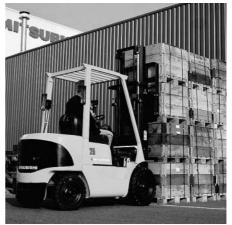
Fig. 1 Counterbalanced type forklift truck
