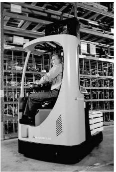
Fig. 2 Reach type forklift truck
