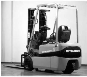
Fig. 8 Rear drive 3-wheel electric counterbalanced forklift truck
