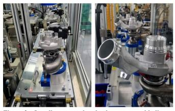
Figure 2 Locally-procured turbocharger assembly line
