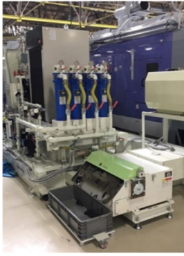
Figure 7 Paperless and environmentally-friendly coolant device dedicated for use with water-soluble coolant
