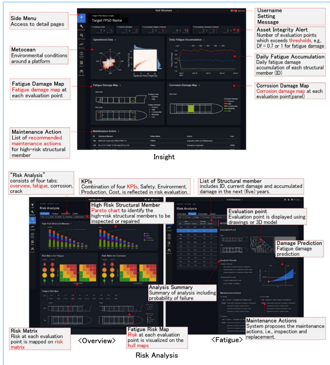
Figure 7 Example of asset integrity management dashboard: hull structure
