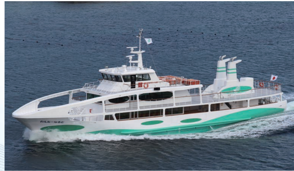
旅客船 S6R2-T2MTK3Lx2 736kW/1406rpmx2 FEG130TH(6D16-MPT)x2 130kVA/1800rpmx2
