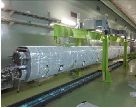
(a) Cold mass of STF2 cryomodule
