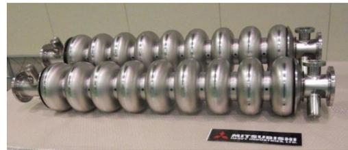
Figure 6: TESLA-shape cavities.
