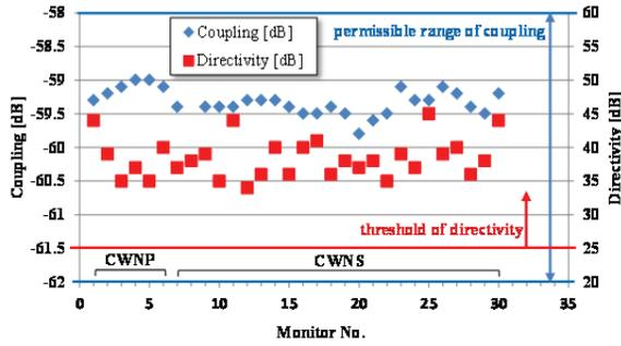
Figure 5: Coupling and directivity of RF monitors.
