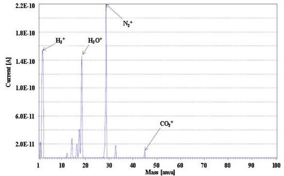
Figure 8: Residual gas analysis of the waveguide unit of CWNS (1<sup>st</sup> shipment).
