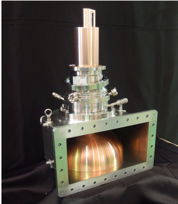
Fine grooves against Multipactoring
