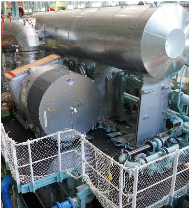
Large-bore low-speed ammonia dual fuel engine with MET66MBII turbocharger
