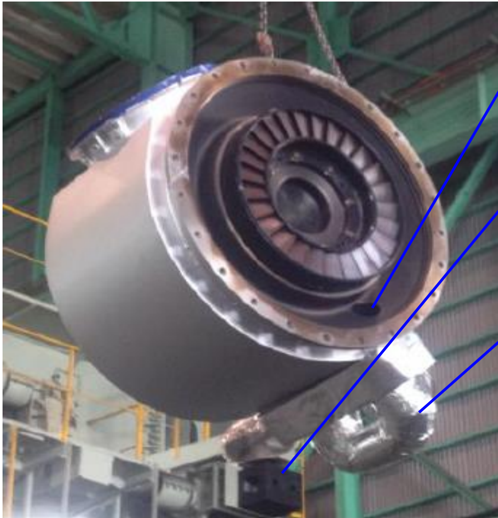
Gas inlet casing assembly with EGB : Mitsubishi MET66MA
