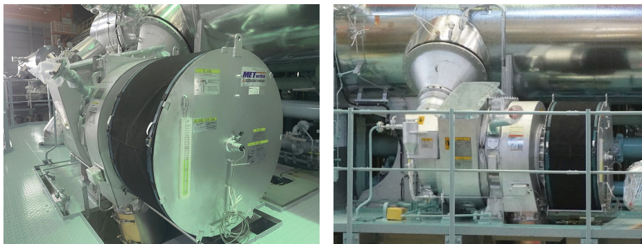
MET turbocharger installed in an engine manufactured by Mitsui E&S Machinery
