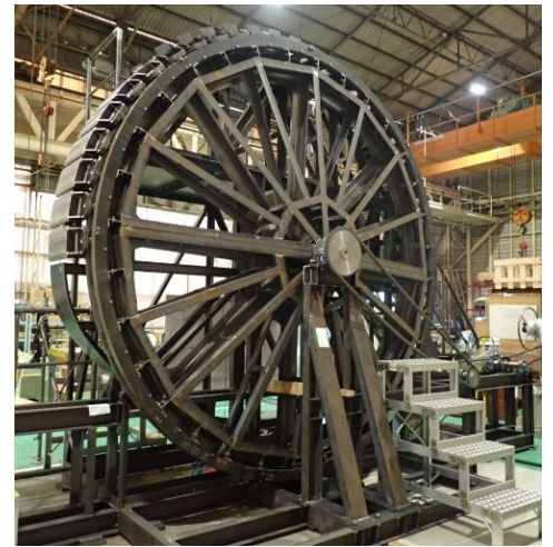
Simulation test apparatus for the new cable drum engine
