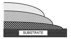
Barrier Coating / PTFE Inhibitive Coating / Metal-Compounds Galvanic Coating / Aluminum-filled Ceramic
