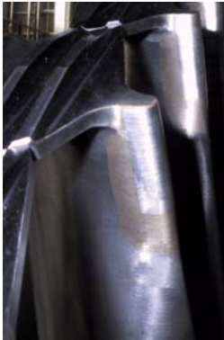
Conventional type (Stellite plate brazing)
