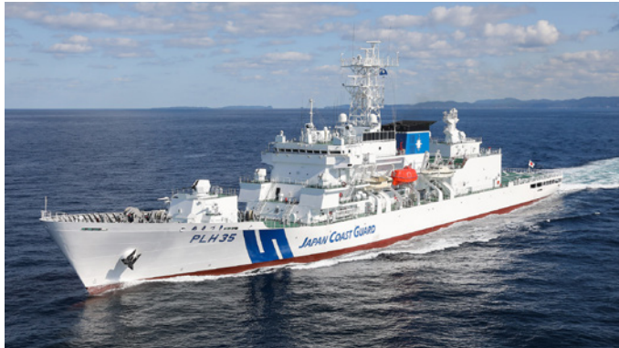
ASAZUKI Patrol Vessel Gross Tonnage ..... 6,500GT Speed ..... 25.5knots or more Length ..... 150 m Shipyard ..... Shimonoseki Breadth ..... 16.8 m
