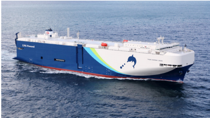
TRANS HARMONY GREEN Ro/Ro cargo ship (LNG-fueled vessel) Gross Tonnage ..... 49,264 GT Speed ..... 19.5 knots Length ..... 195.0 m Shipyard ..... Shimonoseki Breadth ..... 30.6 m
