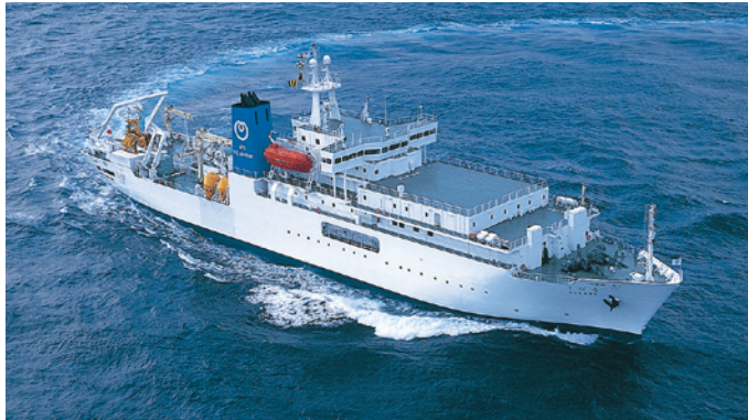
SUBARU Cable Layer Gross Tonnage ..... 9,557 GT Speed ..... 13.2 knots Length ..... 123.33 m Shipyard ..... Shimonoseki Breadth ..... 21.0 m
