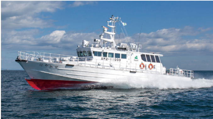
HAYAKAZE Fisheries Patrol Vessel Gross Tonnage ..... 56 GT Speed ..... 35 knots or more Length ..... 26.0 m Shipyard ..... Shimonoseki Breadth ..... 5.4 m
