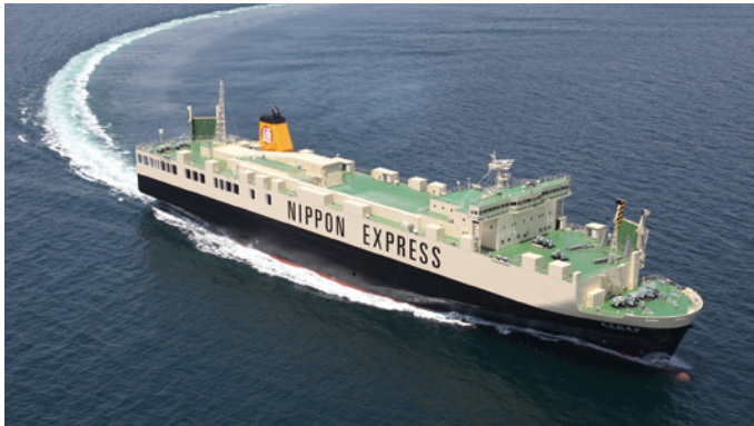
HIMAWARI 8 RO/RO Ship Gross Tonnage ..... 10,626 GT Speed ..... 23.0 knots Length ..... 166.9 m Shipyard ..... Shimonoseki Breadth ..... 27.0 m
