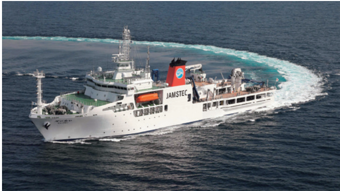
KAIMEI Seabed Research Vessel Gross Tonnage ..... 5,747 GT Speed ..... 12 knots Length ..... 100.5 m Shipyard ..... Shimonoseki Breadth ..... 20.5 m
