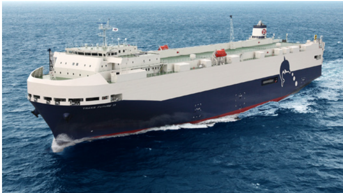
TRANS FUTURE 11 Pure Car Carrier Gross Tonnage ..... 28,775 GT Speed ..... 21.0 knots Length ..... 165.0 m Shipyard ..... Shimonoseki Breadth ..... 27.6 m
