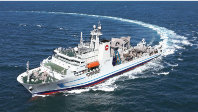
HAKUREI Marine Resource Research Vessel Gross Tonnage ..... 6,283 GT Speed ..... 15.5 knots Length ..... 118.3 m Shipyard ..... Shimonoseki Breadth ..... 19.0 m
