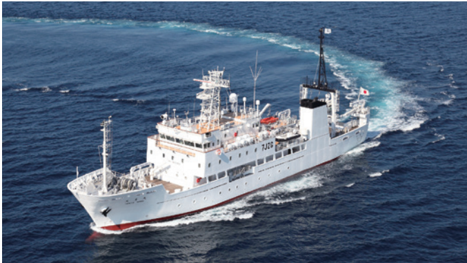
TENYO MARU Fisheries Training Vessel Gross Tonnage ..... 995 GT Speed ..... 12 knots Length ..... 64.67 m Shipyard ..... Shimonoseki Breadth ..... 11.90 m
