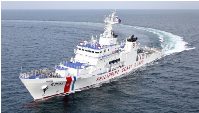
TERESA MAGBANUA Multi-Role Response Vessel Gross Tonnage ..... 2,265 GT Speed ..... 24knots Length ..... 96.6 m Shipyard ..... Shimonoseki Breadth ..... 11.5 m
