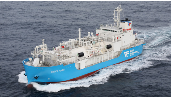
KEYS Azalea Gross Tonnage ..... 4,744 GT Speed ..... 12.0 knots Length ..... 82.4 m Shipyard ..... Shimonoseki Breadth ..... 18.2 m
