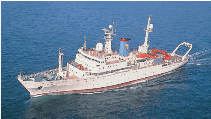
HAKUHO MARU Ocean Research Vessel Gross Tonnage ..... 3,991 GT Speed ..... 16 knots Length ..... 100.0 m Shipyard ..... Shimonoseki Breadth ..... 16.2 m
