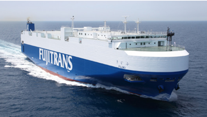
FUJIKI RO/RO Ship Gross Tonnage ..... 15,986 GT Speed ..... 23.0 knots Length ..... 167.0 m Shipyard ..... Shimonoseki Breadth ..... 30.2 m
