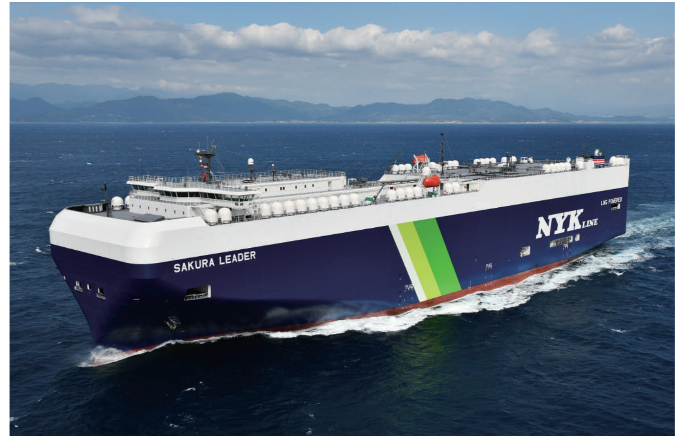
"SAKURA LEADER," the first LNG-fueled pure car carrier built in Japan
