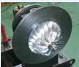
New compressor impeller
