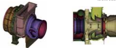
Performance enhanced by rectifying the flow within the casing through improvement of the turbine blade
