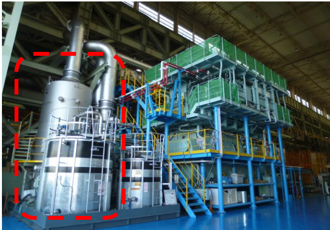
Overview of EGR system in 4UE-X3 (1 st generation)
