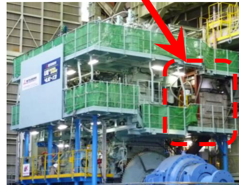
On-engine EGR system (2 nd generation)
