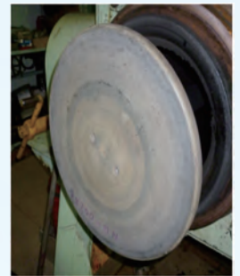
New valve with a weld overlay of heat-resistant steel
