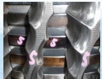
Photo of piston ring after slow steaming
