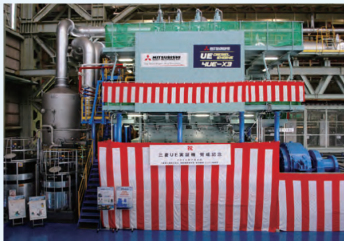
4UE-X3, a full-scale or low-speed diesel test engine
