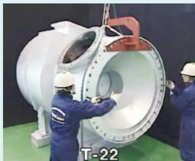
Screw 2 lifting screws(T-22) & lift slowly using a cable with chain block.
