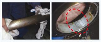
Case in which the journal bearing broke while the rotor was being pulled out because of corrosion and scratches on the surface of the rotor guide tube
