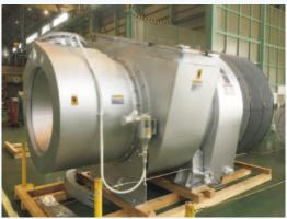
MET Turbocharger mounted on a 12X92DF engine
