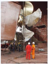
5,000-TEU container ship managed by MSC (Cyprus) on which a propeller retrofit was performed
