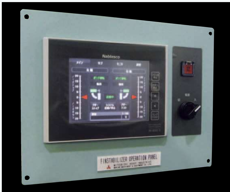
The operating panel for the new control system
