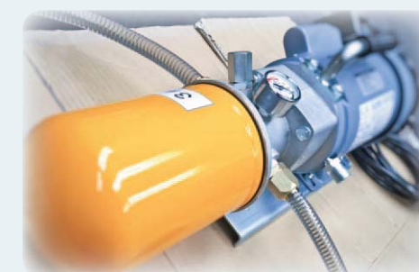
Offline filter exterior
