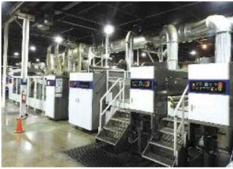
MHI's Evol is a high-speed flexo folder-gluer that boasts fast set ups, quick ink changing and consistent stacking.
