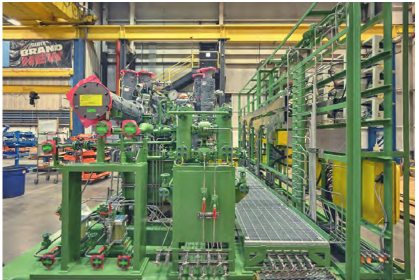
This compressor package for a Middle Eastern oil refinery features an instrument rack with transmitters for local monitoring and a walkway platform for maintenance access. Also included are fan-cooled air-to-air heat exchangers for cooling between compressor stages. Courtesy of FS-Elliott.
