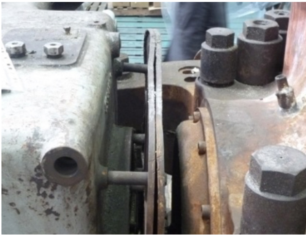
Figure 4. Damaged baffle plate.
