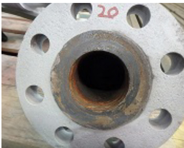
Figure 3. No serration on the flange.
