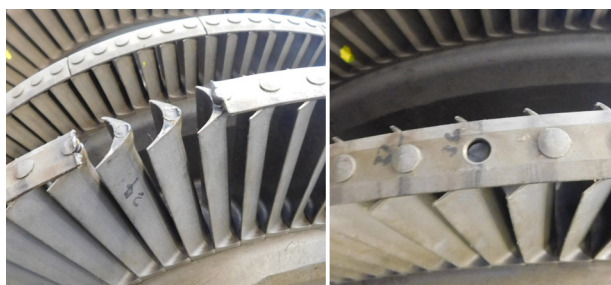
Figure 2. Missing shroud band (left) and tenon (right) found after shutdown.
