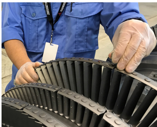
Figure 3. Tenon UT inspection of the subject rotor.
