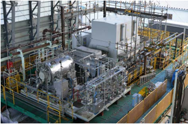
Figure 4. Compressor for pipeline – 37 MW motor-compressor string on test stand in Norway.
