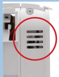
Sensor for indoor temperature and humidity
