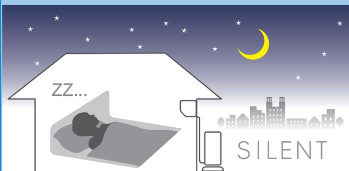
When Silent operation is set, the maximum pressure level of the outdoor unit will be 3dB(A) lower than standard nominal level (45dB(A) or less). The compressor speed is set at a lower range than that of nominal operation, operating at 60% of nominal capacity. Maximum fan speed of outdoor unit is set lower than nominal operation.
