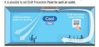
User can position panels by using the remote controller only (RC-EX3A, RCN-TC-5AW-E2) when Draft Prevention Panel is available.
