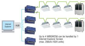
Users can manage up to 1024 units by connecting the four devices!
