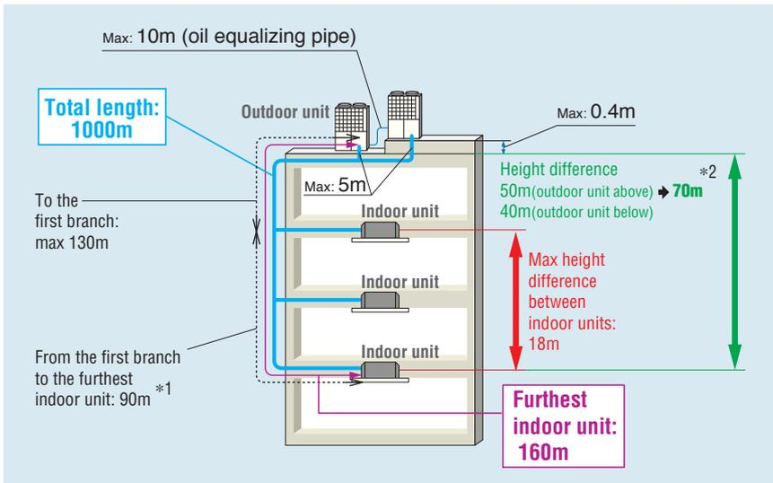
\*1 The difference between the longest and the shortest indoor unit piping from the first branch must be within 40m. (MAX85m)
