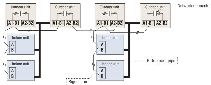
The maximum number of indoor units that can be connected in a system is 128 and it is possible to configure outdoor units and/or indoor units as an outdoor or indoor unit group connected with each other with two wires.
