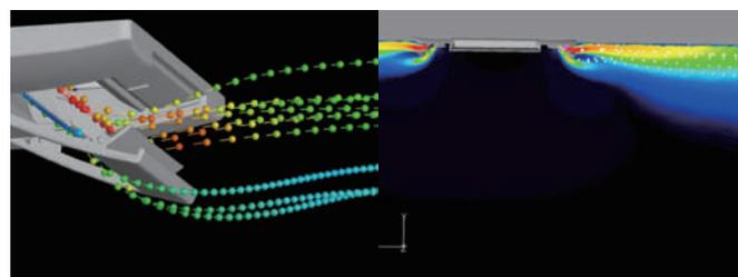
Draft Prevention Panel provides a comfortable airflow without any draft feeling. Whether cooling or heating a room, the remote control can be used to instantly suppress any warm or cool drafts. This accurately assists how air flow is directed out of the indoor unit.
