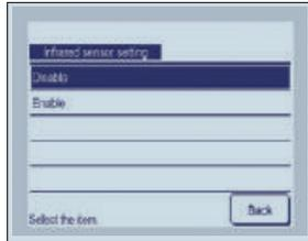
Select [Enable] / [Disable] for the motion sensor of the indoor unit connected to the R/C.
