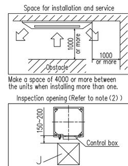
Make a space of 4000 or more between the units when installing more than one.
