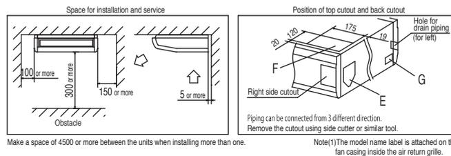
Make a space of 4500 or more between the units when installing more than one.
