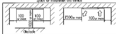
Make a space of 3000 or more between the units when installing more than one.
