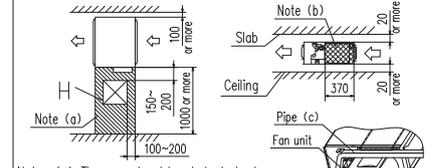
Notes (a) There must not be obstacle to draw out fan unit. For fan unit maintenance, refer to the service manual.
