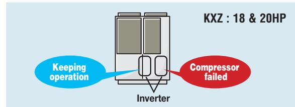
This operation is an emergency measure for a limited time and a necessary repair should be done as soon as possible.
