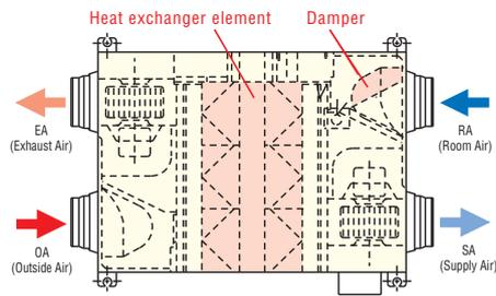
Principle of operation (simple ventilation)
