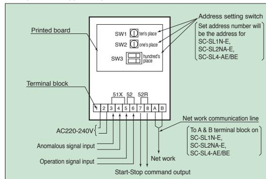
An SC-SL2NA-E performs the start/stop control, monitoring and mode setting of up to 64 units. It is a high quality air conditioner control system that allows up to 64 indoor units to be freely grouped into 1 to 16 groups.
