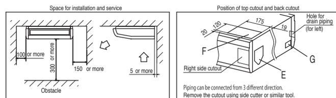
Make a space of 5000 or more between the units when installing more than one.
