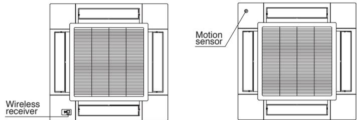
\*Wireless receiver and Motion sensor can be installed to the position as shown
