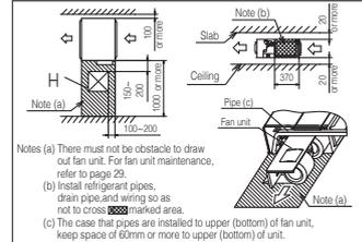
Notes (a) There must not be obstacle to draw out fan unit. For fan unit maintenance, refer to page 29.
