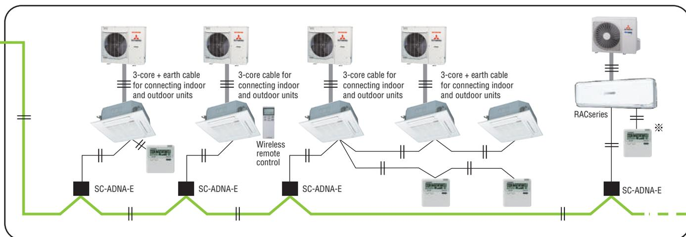
※ SC-BIKN2-E is necessary to connect to wired remote controller.
