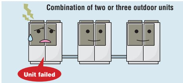
In the event that one compressor has a failure, the unit will keep operating with the other good compressor.
