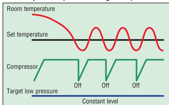
VTCC adjusts the target pressure of the refrigerant cycle in the outdoor unit automatically according to the demand of the indoor units in partial load conditions. These smooth adjustments ensure an optimal capacity usage of the indoor units as well as maximised energy savings. Ultimately this also increases comfort for the user.
