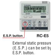
External static pressure (E.S.P.) can be set by E.S.P. button.
