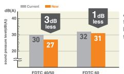
Adopting new turbo fan and improving new heat exchanger enable to reduce noise.
