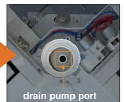
Clean up the area around the drain pump port.
