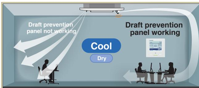
User can position panels by using the remote controller only (RC-EX3A, RCN-TC-5AW-E2) when Draft Prevention Panel is available.
