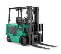
These forklifts have cargo handling equipments such as a mast and a fork, and have a weight attached the rear for counterbalancing the load.
