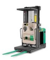
These forklifts have a structure that enables the fork to slide forward (reach) for loading and unloading operations. They bring loads inside when they operate for transport.
