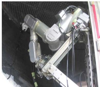
Weld repair robot for steam generator nozzle
