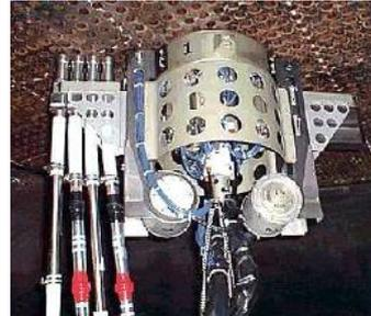
**Inspection robot for SG heat transfer tube**
